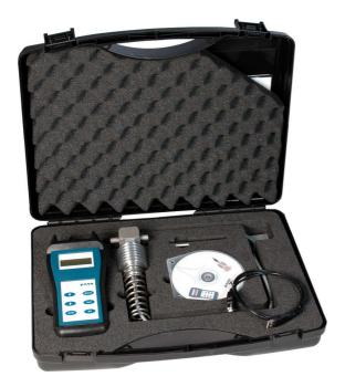
EPM-Peak is a lightweight, battery powered hand held portable device, designed to measure the maximum value of cylinder pressure on 4-stroke diesel engines.
